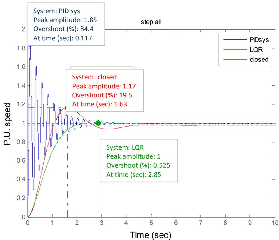
**Fig.8 Closed loop, PID and LQR Step response**
