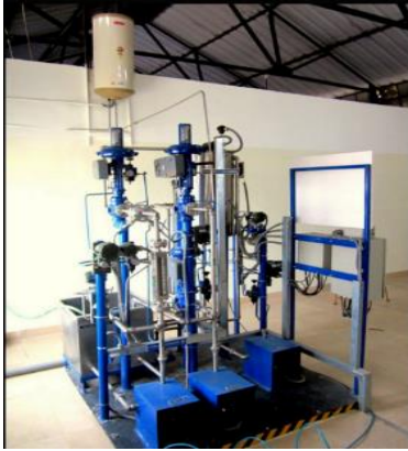
Figure. 1 Real-time CSTR Plant
