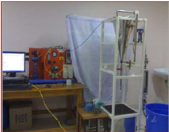
Figure 1: Real time experimental setup of conical tank
