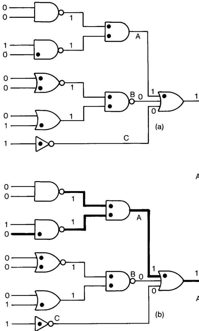
Figure 1. Critical Path Tracing in a Fanout-Free Circuit
