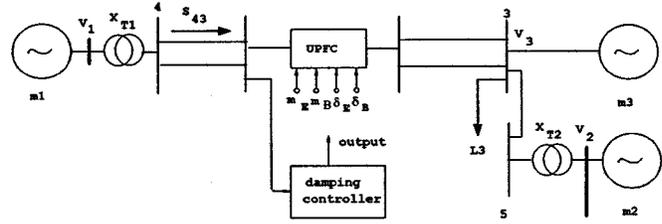
Fig. 7. The example power system.
