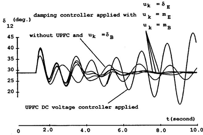
Fig. 8. Non-linear simulation of the three-machine example power system installed with a UPFC.
