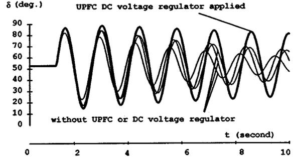
Fig. 5. Non-linear simulation to test the effect of UPFC control on system oscillation damping.
