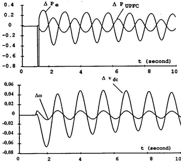
Fig. 6. Non-linear simulation with UPFC installed.
