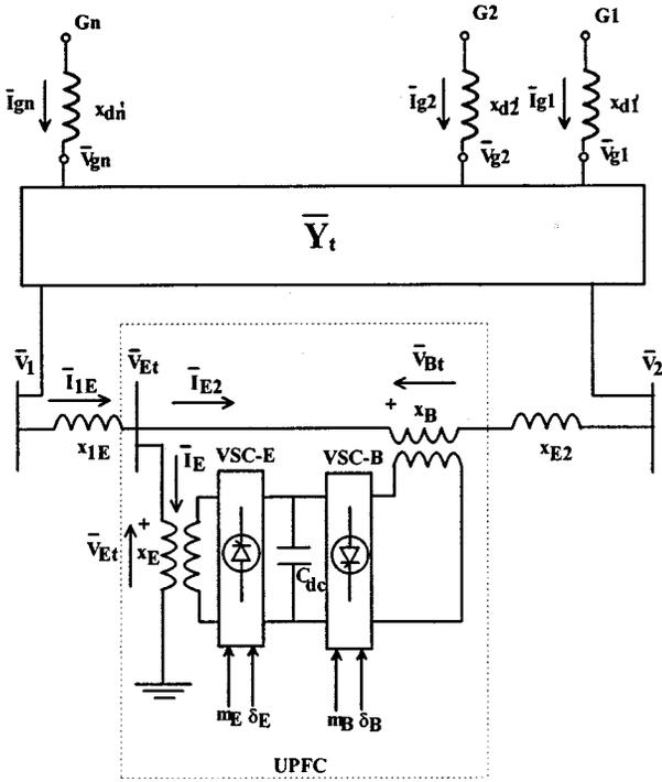
Fig. 3. An  $n$ -machine power system installed with a UPFC.
