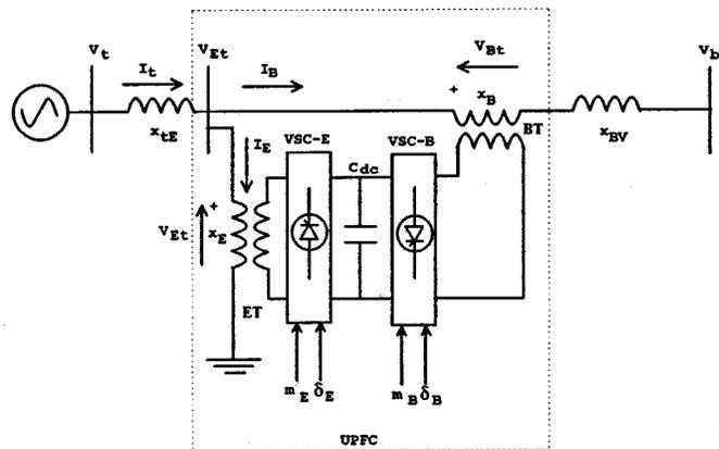
Fig. 1. A UPFC installed in a single-machine infinite-bus power system.
