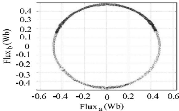
(b) Stator flux linkage of FEV-DTC
