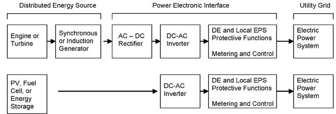
Fig. 1. DE system and PE interface block diagram.
