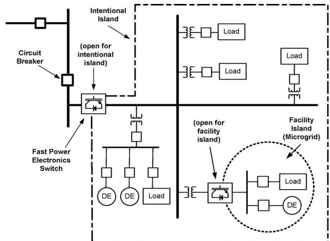
Fig. 4. Intentional island and microgrid example.
