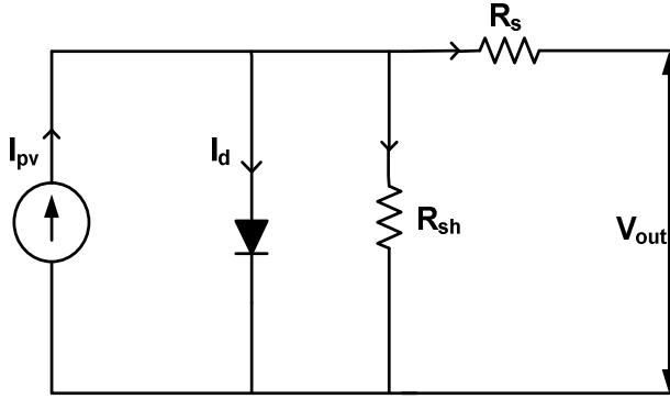
Fig.1. Electrical equivalent circuit of PV cell.
