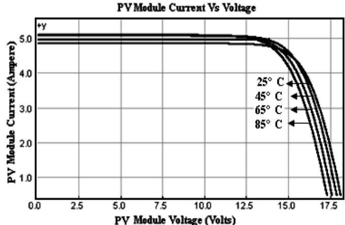
Fig. 3. Current versus voltage at constant solar radiation  $G = 1000 \text{ W/m}^2$ .
