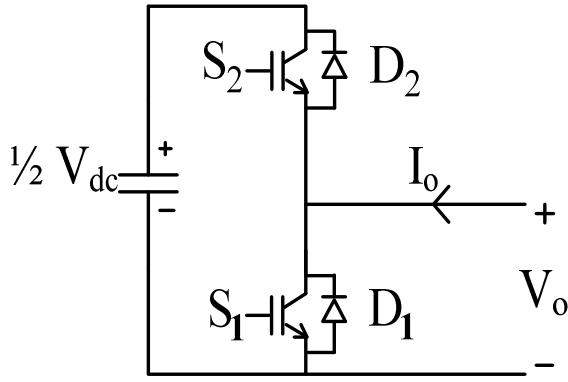
Fig. 4. Structure of one sub-module.
