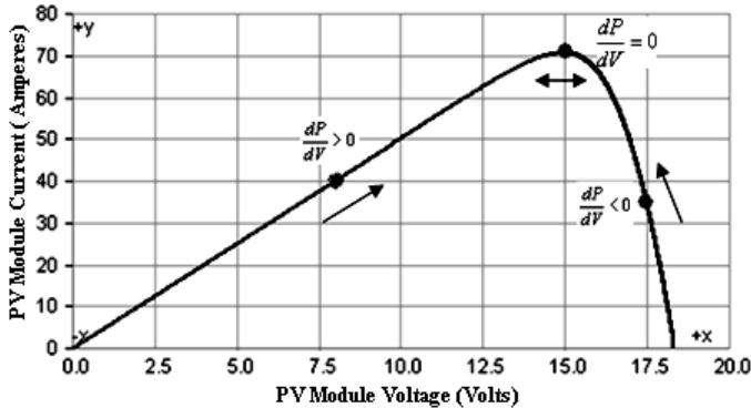
Fig. 7. P-V characteristics of the module.
