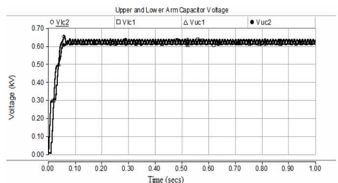
Fig.9 Capacitor voltage across lower and upper arm.
