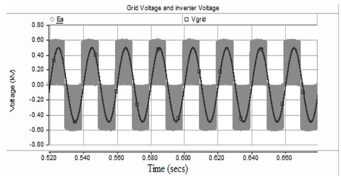
Fig.14 Grid voltage and MMC output voltage.
