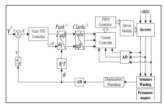
Figure 2. Configration of the PMLSM system
