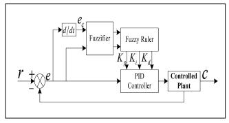
Figure 3. Configration of the fuzzy PID control
