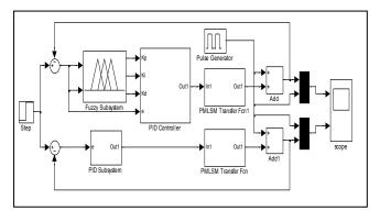
Figure 4. The simulation model of fuzzy PID controller
