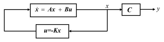
Fig. 3 Linear Quadratic Regulator Structure
