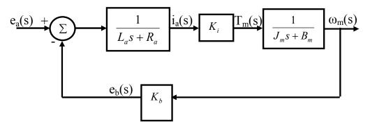
Fig. 2- DC-Motor System Block Diagram for speed (Plant System)
