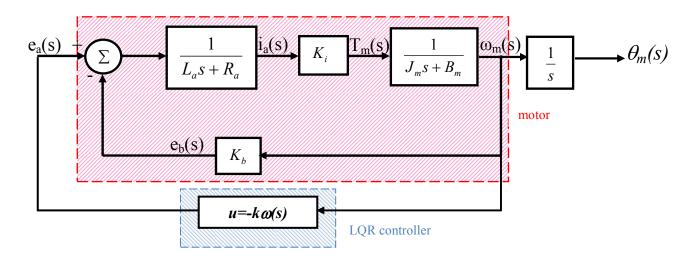
Fig. 4- DC-Motor System with LQR
