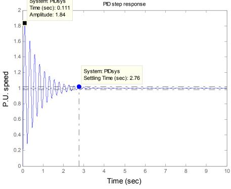
Fig.6 PID Step Response
