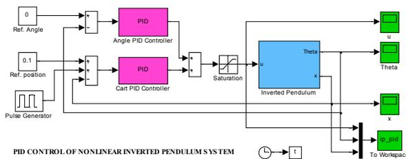
Figure 2. PID Control of Nonlinear Inverted Pendulum-Cart System.
