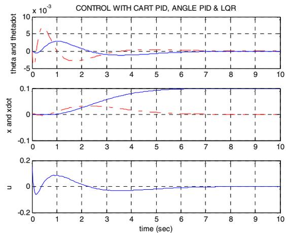
Figure 5. Responses of pendulum angle  $\theta$ , angular velocity  $\dot{\theta}$ , cart position  $x$ , cart velocity  $\dot{x}$ , and control force  $u$  of nonlinear inverted pendulum system with Angle PID, Cart PID & LQR Control.
