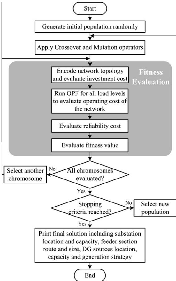
Fig. 1. Flow chart of hybrid GA-OPF optimization approach.
