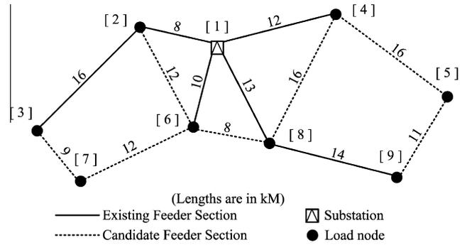
Fig. 3. Test distribution system.
