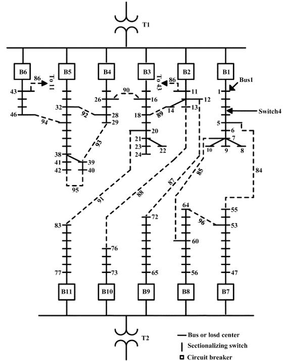
Fig. 4. Typical Taiwan Power Company distribution system topology.
