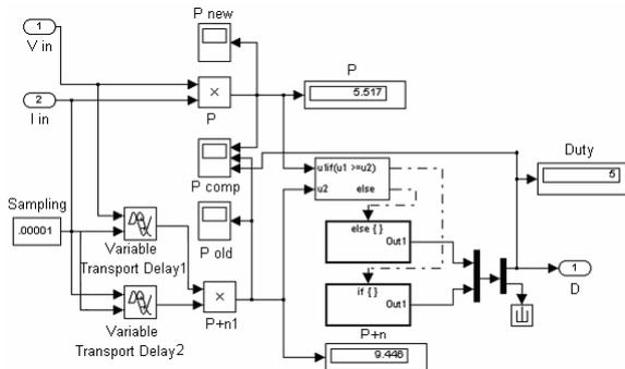
Fig. 8: Block diagram of the P&O algorithm in the Matlab - Simulink.
