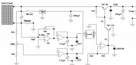
Fig. 15: Electric diagram of prototype to the photovoltaic generator.
