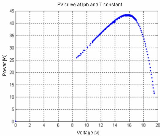
Fig. 13:  $P \times V$  characteristic curve of the solar panel
