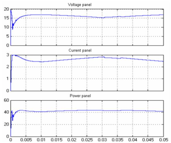
Fig. 10: Output signals of the solar panel with resistive load variable.
