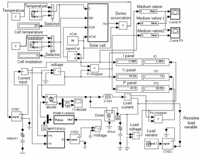
Fig. 9: Complete diagram of the photovoltaic converter with MPPT algorithm.
