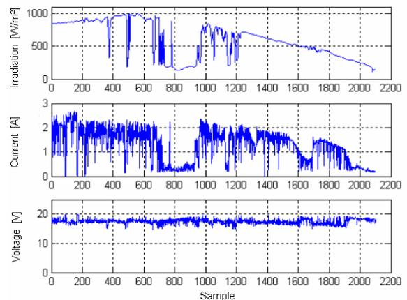
Fig. 16: Measurements of solar irradiation, current and voltage of input power converter.
