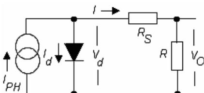
Fig. 2: Simplified equivalent circuit of the solar cell.
