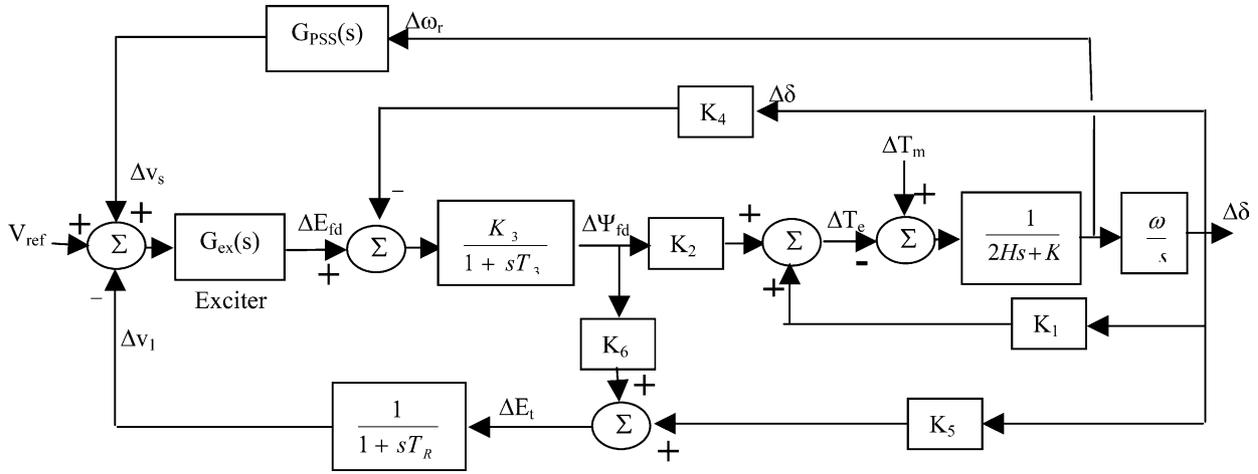
Fig. 2. Block diagram representation with AVR and PSS.
