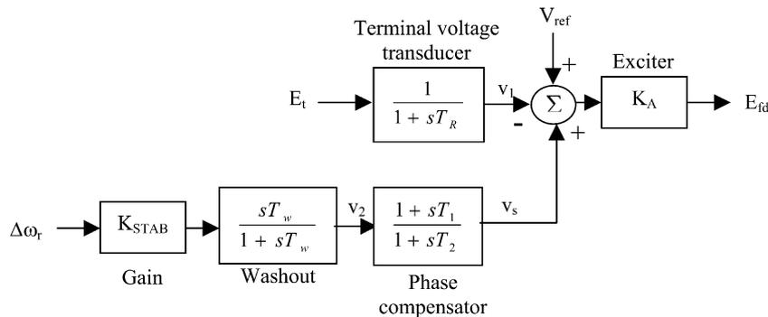
Fig. 3. Thyristor excitation system with AVR and PSS.
