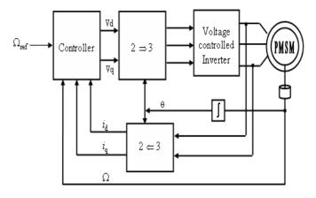
Fig. 2. System configuration of Backstepping control
