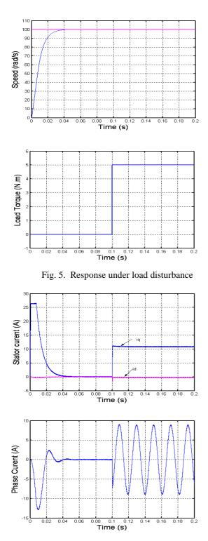
Fig. 6. Stator current under load disturbance
