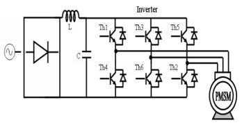
Fig. 3. Basic three-phase voltage-source converter circuit
