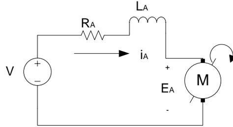
Figure 2: Electrical Equivalent Circuit of Motor Armature.
