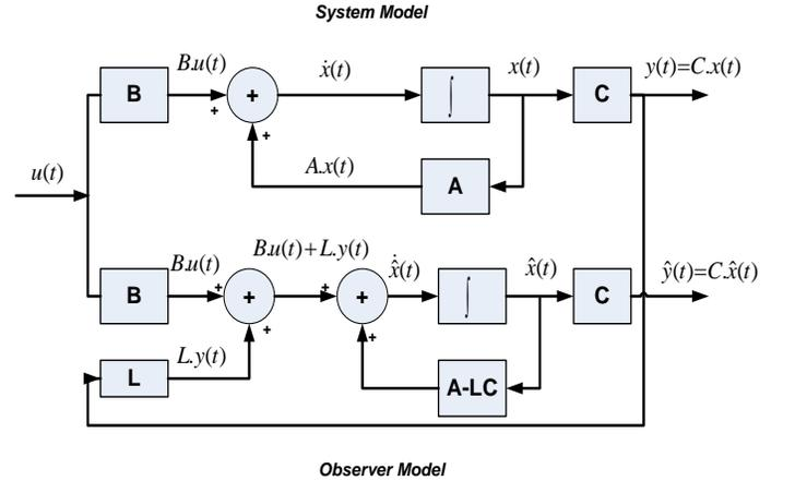
Figure 1: Block Diagram of System and Observer Models.
