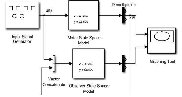
Figure 3: Simulink Block Diagram for the DC Motor Model and the Full Observer Model.
