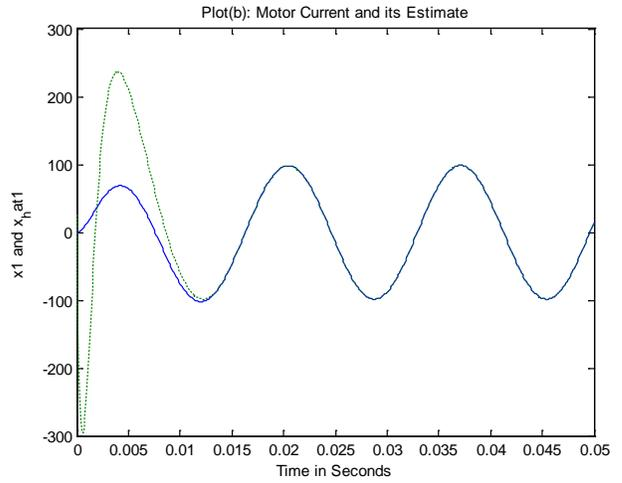
Figure 4: (a): Input pulse Voltage, (b)-(d): Plots of armature current, shaft position, and motor angular speed and their respective estimates, as produced by the observer system..
