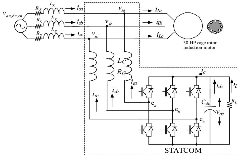
Fig. 1. Schematic of shunt compensated induction motor.
