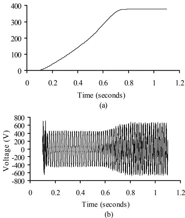
Fig. 5. Starting response of a high power induction motor with a STATCOM-based compensation technique (a) speed of the induction motor and (b) phase  $a$  voltage  $v_{s_a}$  across the motor winding.
