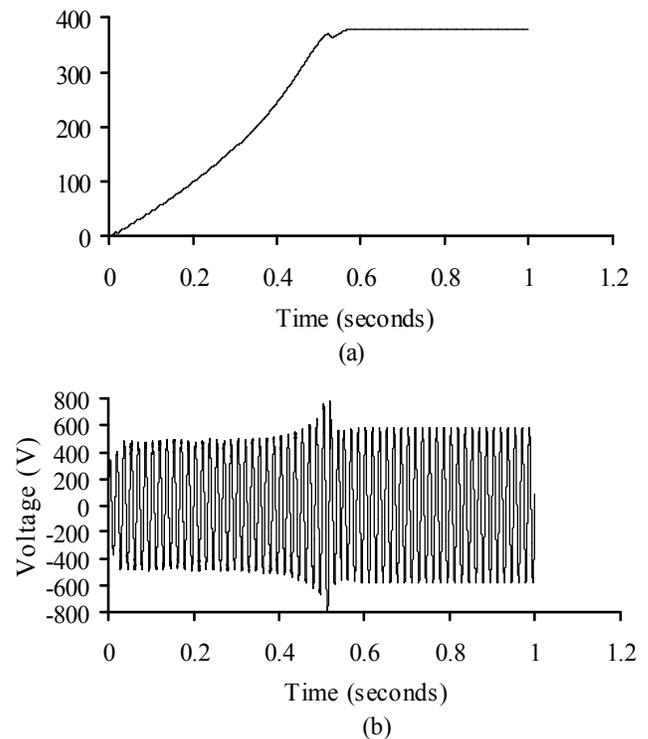
Fig. 7. Starting response of a high power induction motor with the SSSC-based compensation technique (a) speed of the induction motor and (b) phase  $a$  voltage  $v_{s_a}$  across the motor winding.
