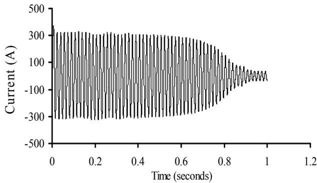
Fig. 4. Starting current for the phase  $a$  winding ( $i_{L_a}$ ) of a high power induction motor without any compensation.
