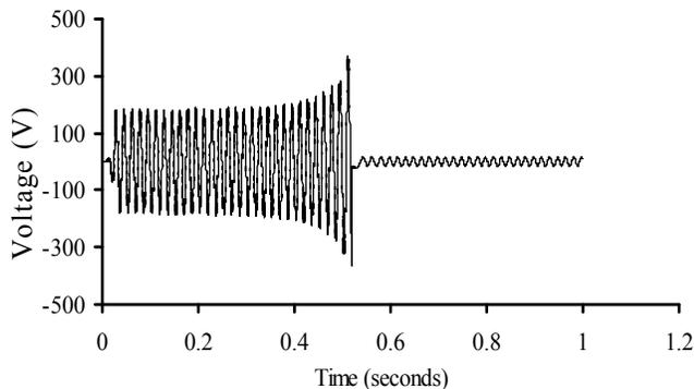
Fig. 9. Injected voltage in series with the motor.
