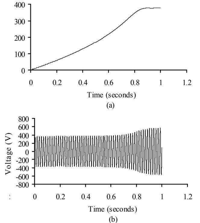
Fig. 3. Starting response of high power induction motor without compensation (a) speed of the induction motor and (b) phase  $a$  voltage  $v_{sa}$  across the motor winding.
