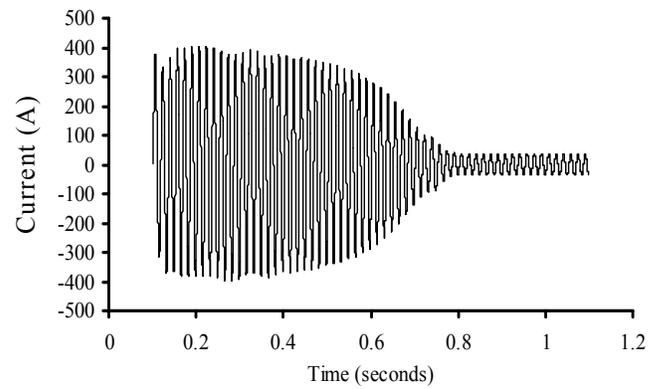
Fig. 6. Starting current for the phase  $a$  winding ( $i_{L_a}$ ) of a high power induction motor with the STATCOM-based compensation technique.
