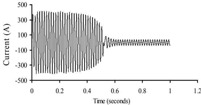
Fig. 8. Starting current for the phase  $a$  winding ( $i_{La}$ ) of a high power induction motor with SSSC-based compensation technique.
