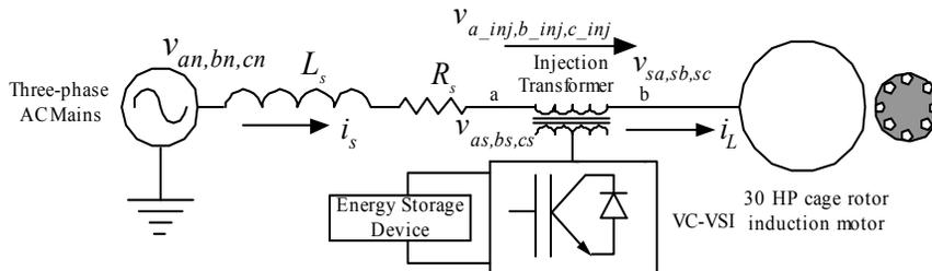
Fig. 2. Single line diagram of an active series compensated induction motor.
