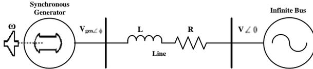
Figure 1: Single line diagram of the power system
