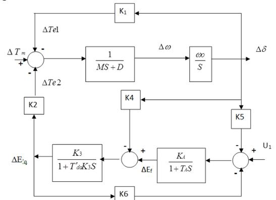
Figure2 : Block diagram of the model power system [8], [9].
