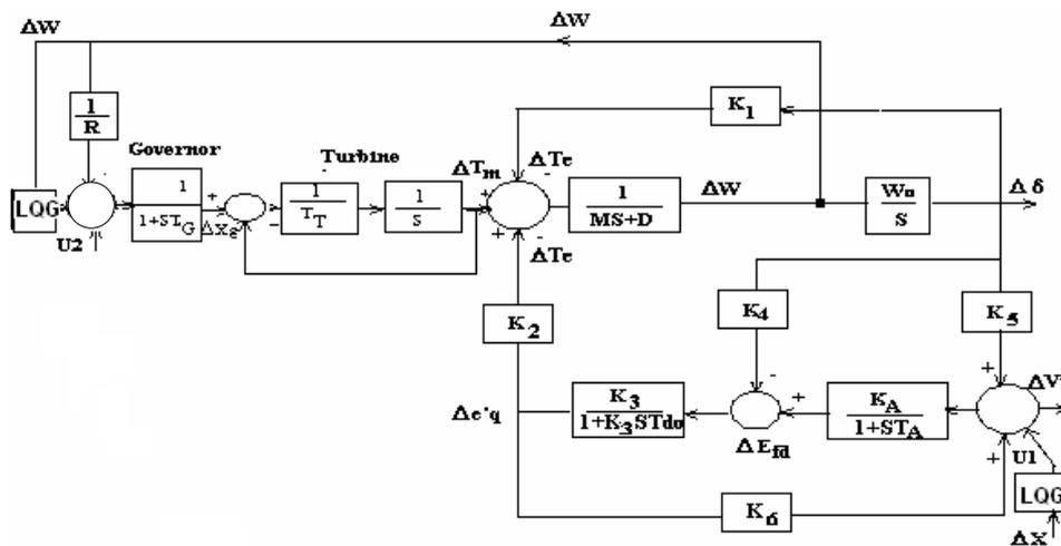
Figure 3: The block diagram of interconnected power system [10].
