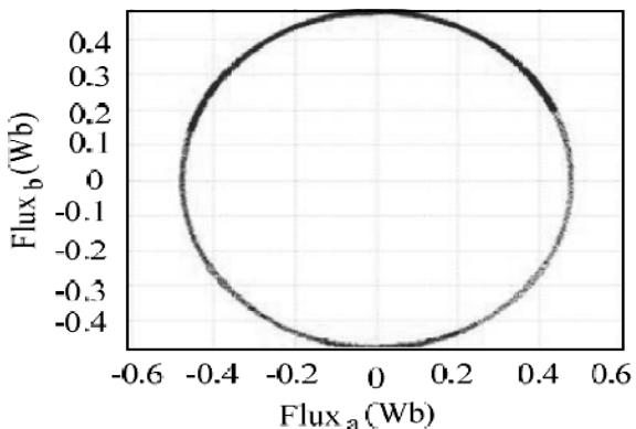
(a) Stator flux linkage of FEV-DTC
