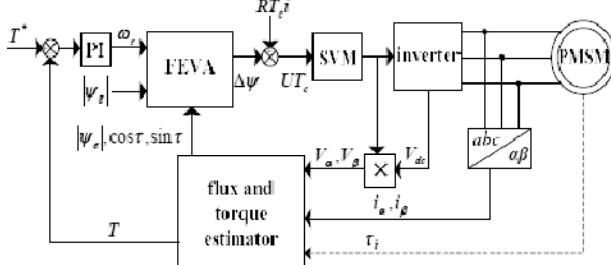
Fig.2 FEVA-DTC system scheme
