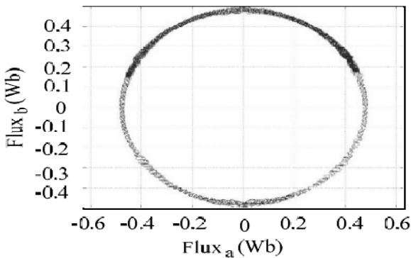
(b) Stator flux linkage of FEV-DTC
