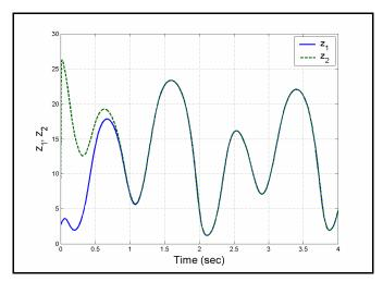
Figure 7. Complete synchronization of the states  $z_1(t)$  and  $z_2(t)$
