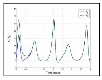
Figure 5. Complete synchronization of the states  $x_1(t)$  and  $x_2(t)$
