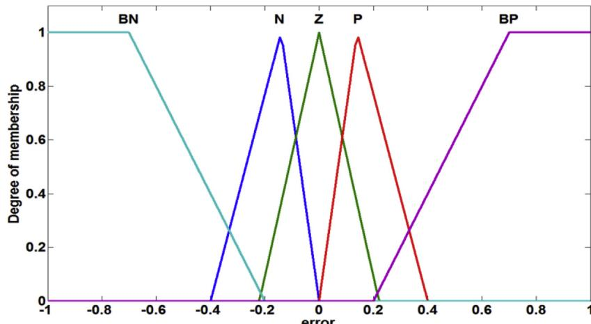
Fig. 7. Fuzzy membership functions for: voltage error, change of error of the rotor voltage, and the output of the DFIG rotor speed FLC estimation.
