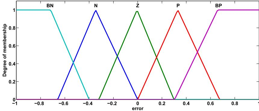
Fig. 4. Membership functions on inputs and output of the FLC wind speed estimator (Revised).
