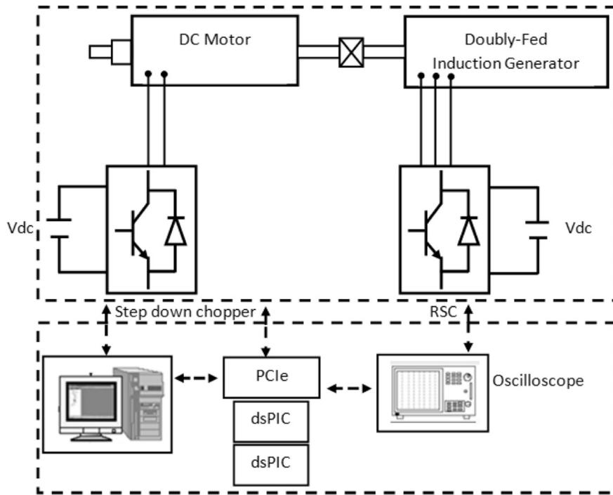
**Fig. 26.** Structure of the experimental test bench of wind emulator.
