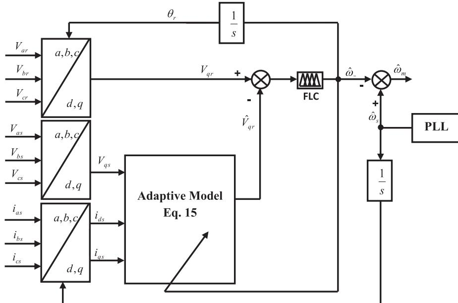
Fig. 5. Schematic blocks of the MRAS based DFIG rotor speed observer (Revised).
