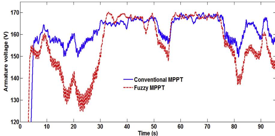
Fig. 30. Armature voltage for both MPPT algorithms.
