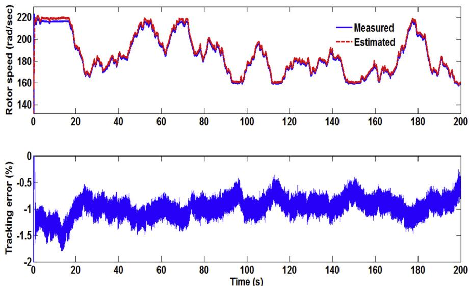
Fig. 17. DFIG rotor speed estimation performance using MRAS.
