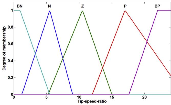
Fig. 11. Membership functions of the tip speed ratio.
