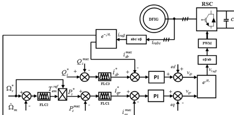
Fig. 2. Block diagram of the overall RSC control scheme.
