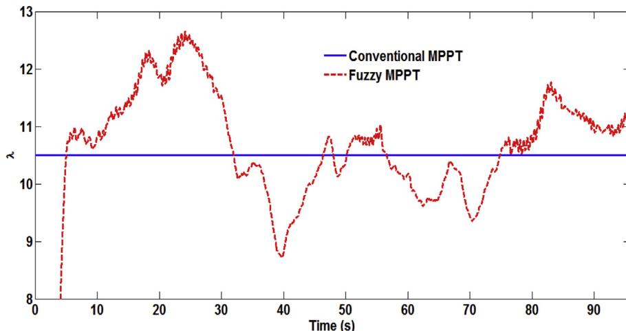
**Fig. 29.** Comparison of the variation of tip speed ratio for both MPPT algorithms.
