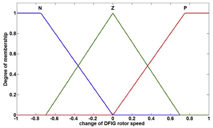
Fig. 14. Membership functions of the change of the DFIG rotor's speed.
