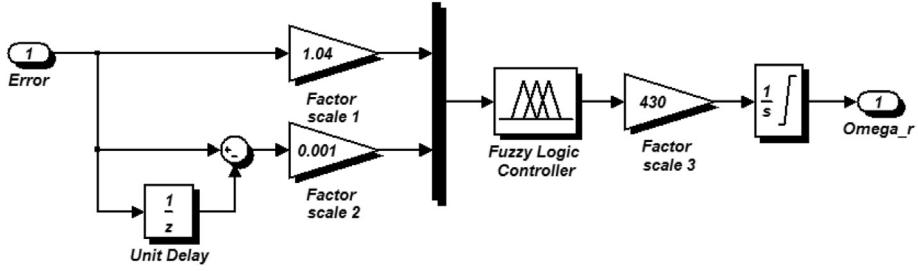
Fig. 6. Structure of fuzzy logic controller of MRAS observer.
