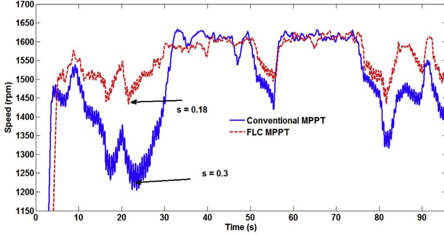
**Fig. 28.** Comparison of the measured speed of the wind emulator for both MPPT algorithms.
