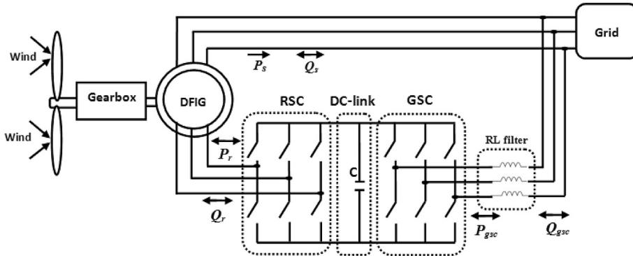
Fig. 1. General scheme of the wind energy conversion system.
