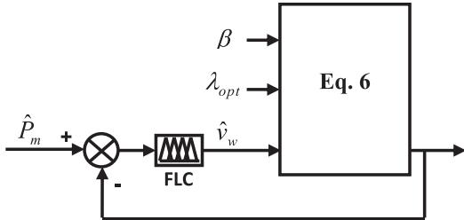
Fig. 3. Fuzzy technique based wind speed estimation (Revised).
