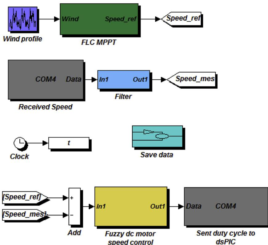
Fig. 25. Simulink scheme of MPPT control using serial communication.
