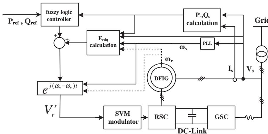
**Fig. 5.** Schematic of the proposed FDPC for DFIG.
