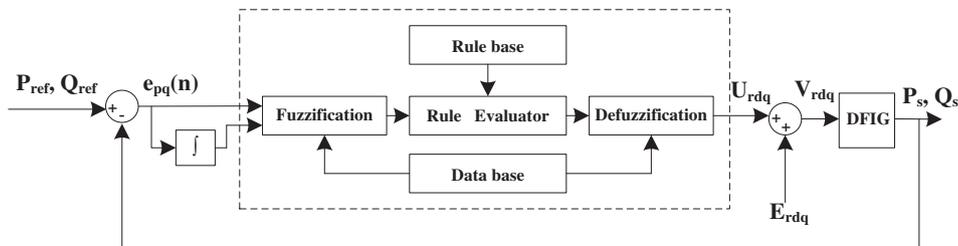
Fig. 3. Structure of FDFPC method.
