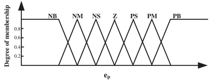
Fig. 4. Fuzzy set of the active power error.
