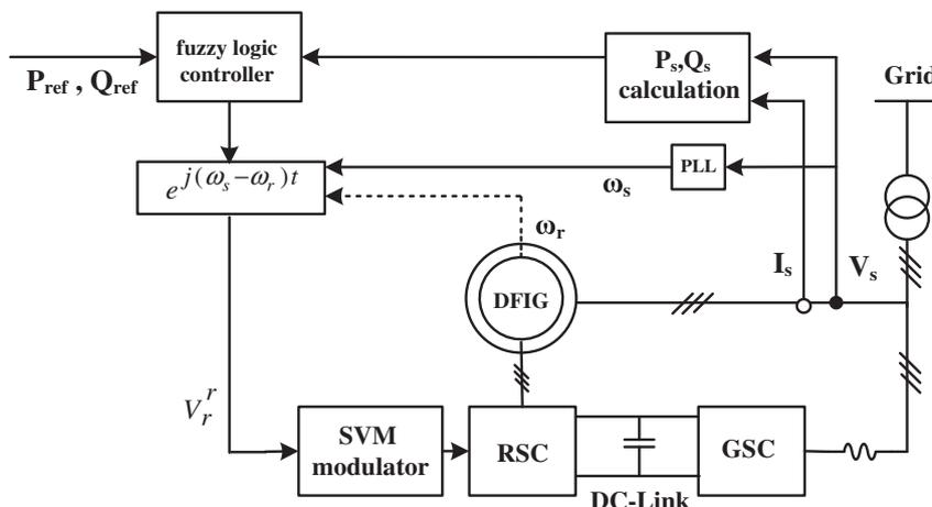
**Fig. 6.** Schematic of the proposed FFDPC for DFIG.
