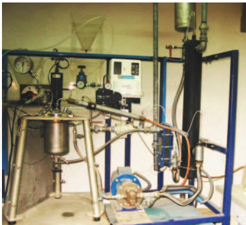
Fig. 2. The esterification reactor used for the experiments.
