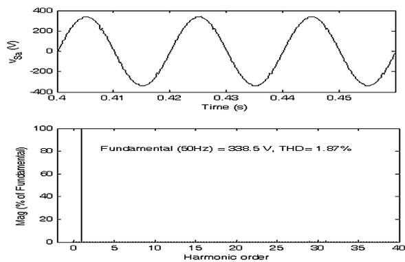
Fig. 12. Voltage at PCC with compensator.
