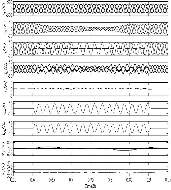
Fig. 8. Performance of a three-phase three-leg VSC and T-connected transformer-based DSTATCOM for neutral current compensation, load balancing, and power factor correction.
