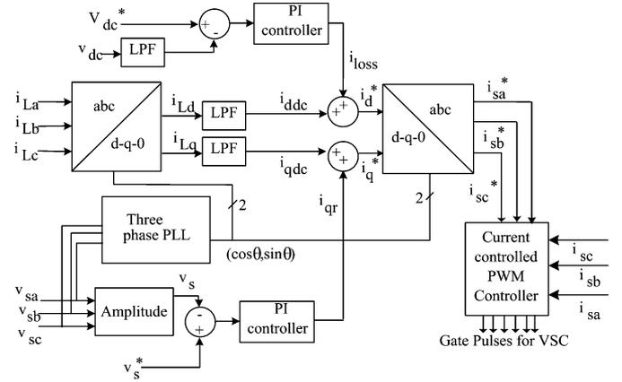
Fig. 4. Control algorithm for the three-leg-VSC-based DSTATCOM in a three-phase four-wire system.
