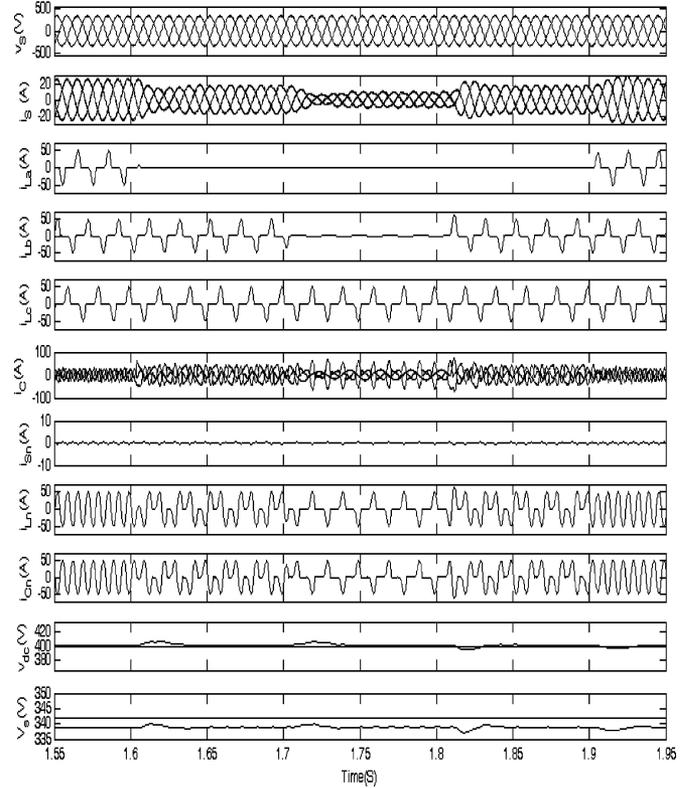
Fig. 9. Performance of a three-phase three-leg VSC and T-connected transformer-based DSTATCOM for neutral current compensation, load balancing, harmonic compensation, and power factor correction.
