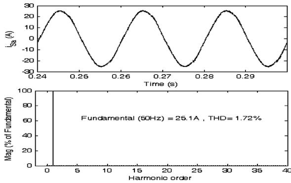
Fig. 11. Source current and the harmonic spectrum.
