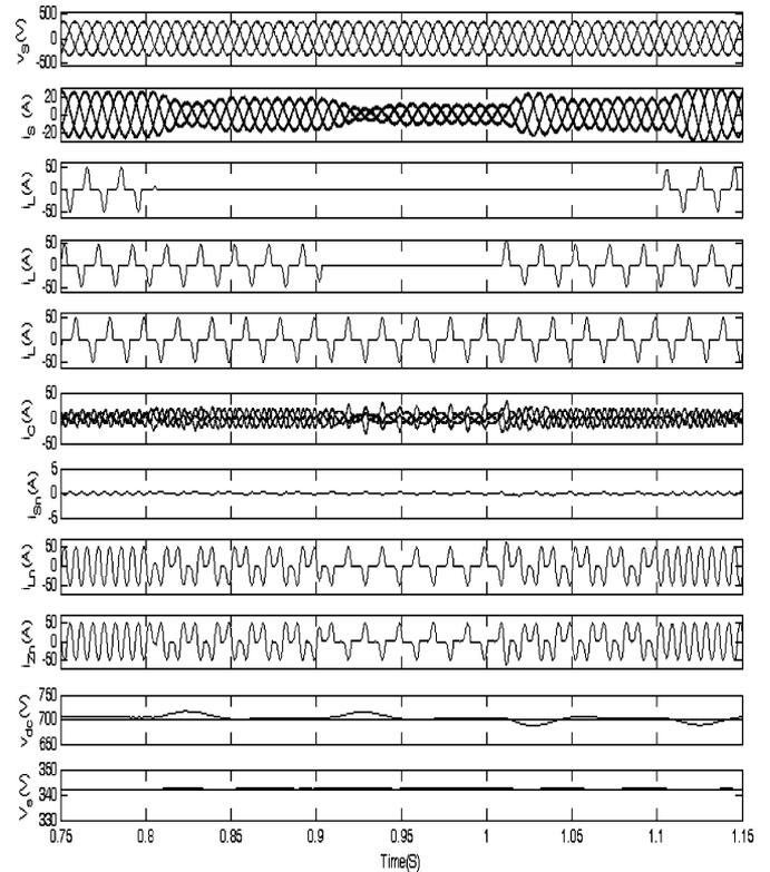
Fig. 7. Performance of a three-phase three-leg VSC and T-connected transformer-based DSTATCOM for neutral current compensation, load balancing, harmonic compensation, and voltage regulation.
