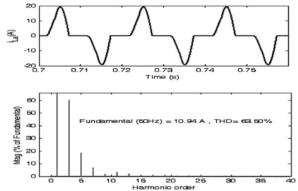
Fig. 10. Load current and the harmonic spectrum.
