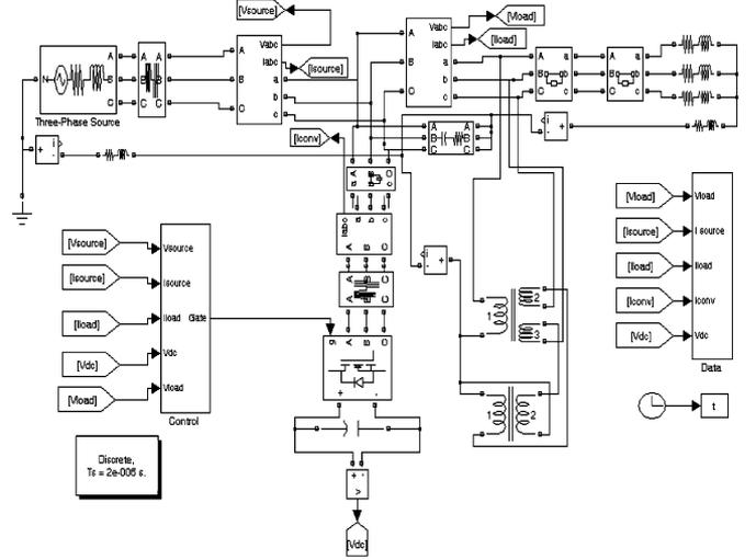
Fig. 5. MATLAB model of the T-connected transformer and the three-leg-VSC-based DSTATCOM-connected system.
