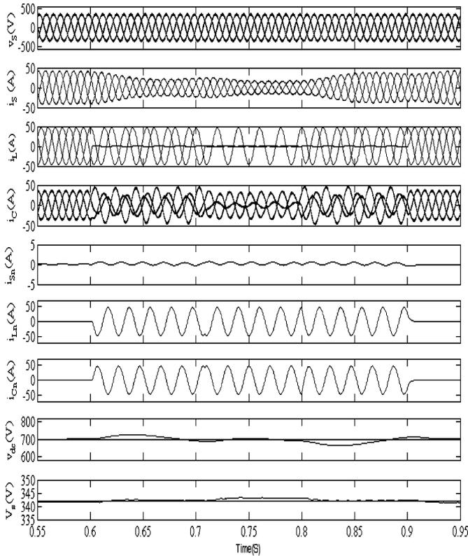
Fig. 6. Performance of a three-phase three-leg VSC and T-connected transformer-based DSTATCOM for neutral current compensation, load balancing, and voltage regulation.
