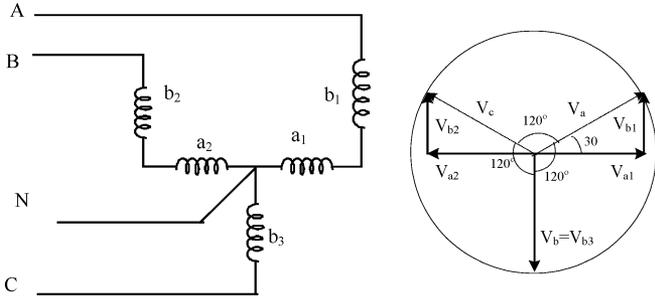
Fig. 3. (a) T-connected transformer and the three-leg VSC. (b) Phasor diagram.
