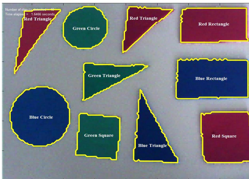
Fig. 11 Results of algorithm on multiple objects.
