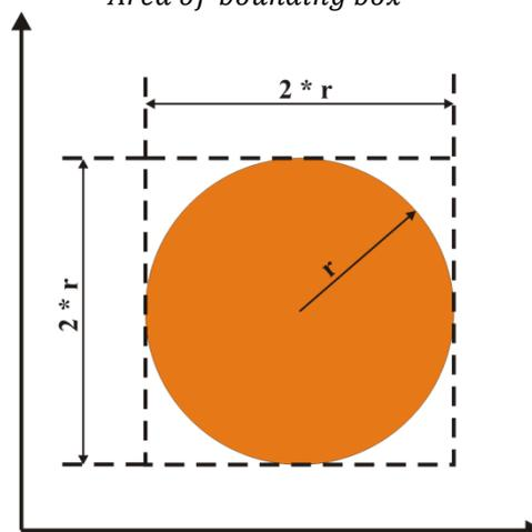
Fig. 4 Bounding box dimensions for a circle.
