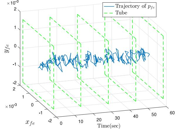
Fig. 5. The error between actual and nominal states lies in a tube.
