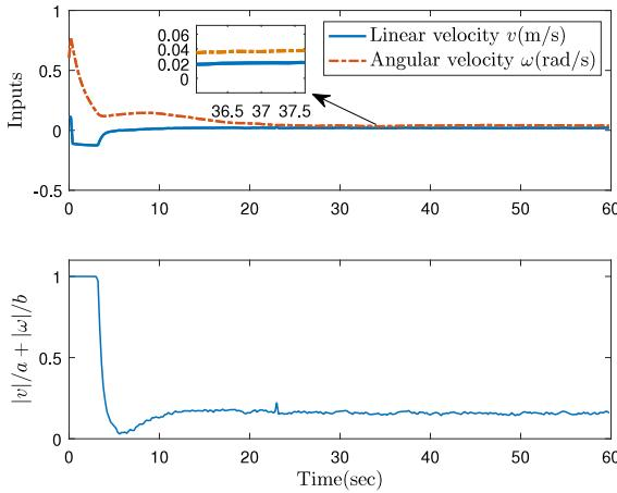
Fig. 11. Control input of NRMPC.
