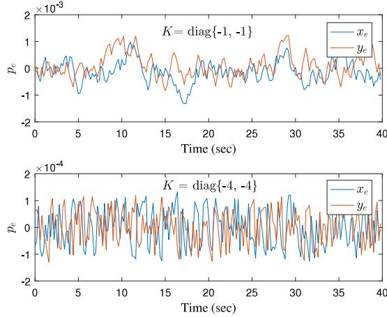
**Fig. 7.** Real-time position deviation from the center of the tube  $p_{fe}$  with different feedback gains.
