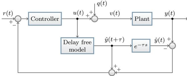
Fig. 1. Standard Smith predictor structure.
