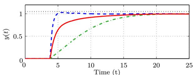
Fig. 4. Step response of the system (26) in closed-loop using the controller designed as proposed: in this paper (dashed line), the method in Palmor and Blau (1994) (solid line), and the one in Mozelli and Souza (2016) (dash-dot line).
