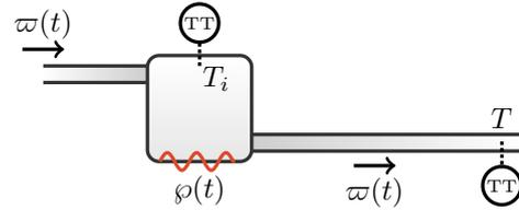
Fig. 3. Water heater adapted from Normey-Rico and Camacho (2007).
