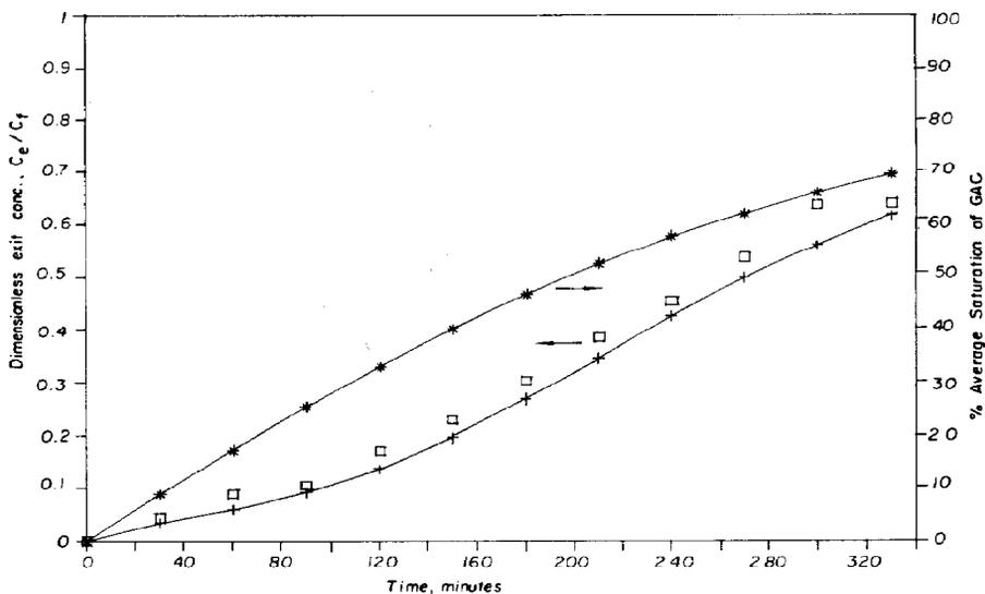
Fig. 13. Fluidized-bed adsorber breakthrough curve with 0.075 kg of  $1.545 \times 10^{-3}$  m  $\phi$  (# 12/14 mesh) GAC:  $\square$  experiment with  $C_f = 2.02$  mol/m<sup>3</sup>,  $\bar{u} = 0.0075$  m/s;  $-+-$  simulation with  $C_f = 2.02$  mol/m<sup>3</sup>,  $\bar{u} = 0.0075$  m/s.
