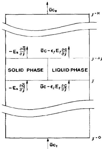
Fig. 1. Schematic representation of the fluidized-bed adsorber.
