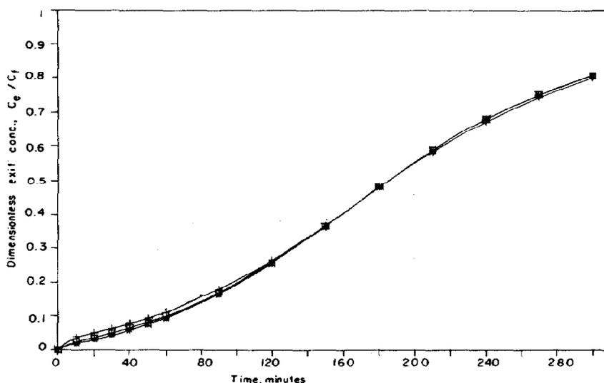
Fig. 6. Sensitivity analysis: effect of the liquid-phase axial dispersion coefficient  $E_l$  on the breakthrough curve;  $+0.3E_l$ ,  $\square$   $1.0E_l$ ,  $*$   $3.0E_l$ .
