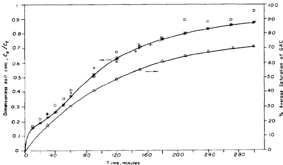
Fig. 9. Fluidized-bed adsorber breakthrough curve with 0.075 kg of  $1.545 \times 10^{-3}$  m  $\phi$  (#12/14 mesh) GAC:  $\square$  experiment with  $C_f = 2.02$  mol/m<sup>3</sup>,  $\bar{u} = 0.0181$  m/s; + experiment with  $C_f = 1.88$  mol/m<sup>3</sup>,  $\bar{u} = 0.0174$  m/s; — \* — simulation with  $C_f = 1.95$  mol/m<sup>3</sup>,  $\bar{u} = 0.0178$  m/s.
