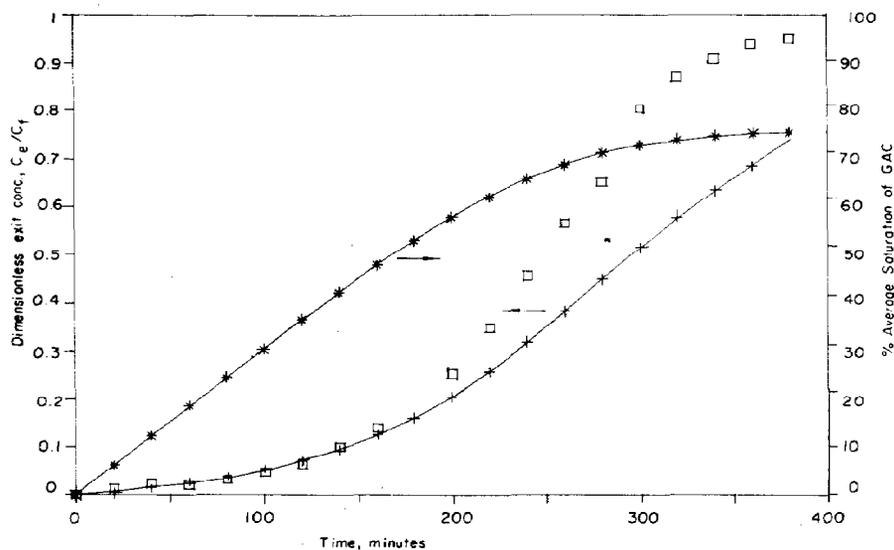
Fig. 15. Fluidized-bed adsorber breakthrough curve with 0.075 kg of  $0.92 \times 10^{-3}$  m  $\phi$  (# 18/20 mesh) GAC: □ experiment with  $C_f=1.88$  mol/m<sup>3</sup>,  $\bar{u}=0.0083$  m/s; -+- simulation with  $C_f=1.88$  mol/m<sup>3</sup>,  $\bar{u}=0.0083$  m/s.
