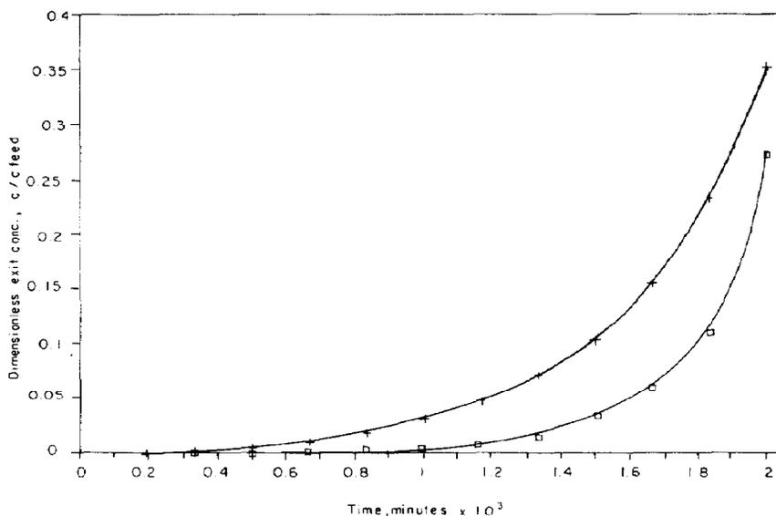
Fig. 7. Sensitivity analysis: effect of the solid-phase mixing coefficient  $E_s$  on the breakthrough curve in a relatively long column (GAC = 0.75 kg); +  $3.0E_s$ , □  $1.0E_s$ .
