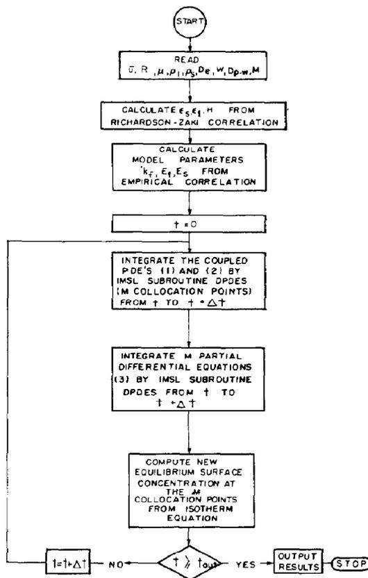
Fig. 2. Algorithm for simulating the fluidized-bed adsorber performance.
