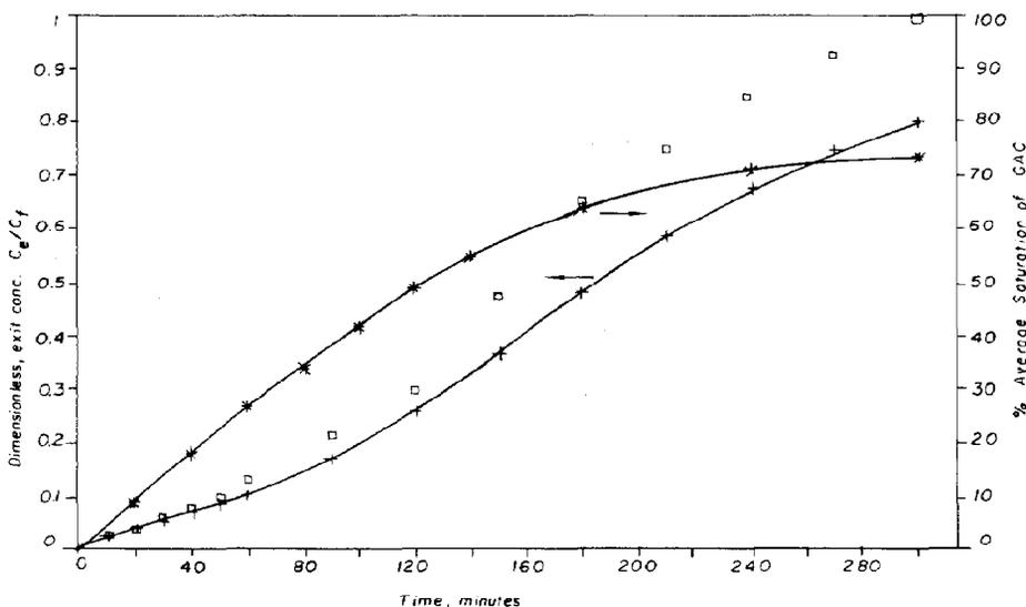
Fig. 14. Fluidized-bed adsorber breakthrough curve with 0.075 kg of  $0.92 \times 10^{-3}$  m  $\phi$  (# 18/20 mesh) GAC: □ experiment with  $C_f=1.41$  mol/m<sup>3</sup>,  $\bar{u}=0.0157$  m/s; -+- simulation with  $C_f=1.41$  mol/m<sup>3</sup>,  $\bar{u}=0.0157$  m/s.
