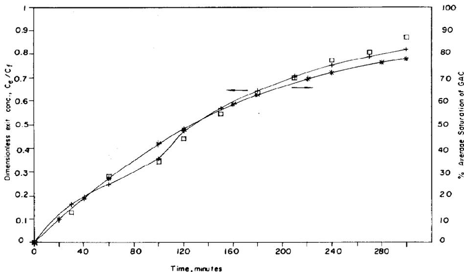
Fig. 12. Fluidized-bed adsorber breakthrough curve with 0.06 kg of  $1.545 \times 10^{-3}$  m  $\phi$  (# 12/14 mesh) GAC:  $\square$  experiment with  $C_f = 1.82$  mol/m<sup>3</sup>,  $\bar{u} = 0.0115$  m/s;  $-+-$  simulation with  $C_f = 1.82$  mol/m<sup>3</sup>,  $\bar{u} = 0.0115$  m/s.
