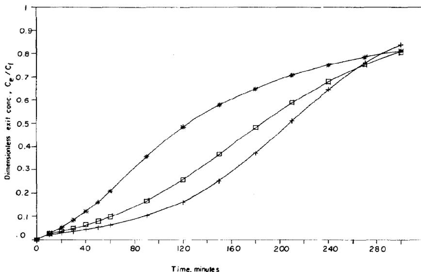
Fig. 3. Sensitivity analysis: effect of the intraparticle transport coefficient  $D_e$  on the breakthrough curve; \* $0.3D_e$ ,  $\square$   $1.0D_e$ ,  $\times$   $3.0D_e$ .
