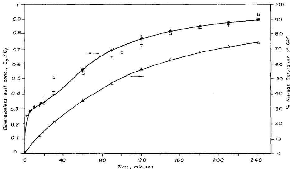
Fig. 11. Fluidized-bed adsorber breakthrough curve with 0.04 kg of  $1.545 \times 10^{-3}$  m  $\phi$  (# 12/14 mesh) GAC: + experiment with  $C_f = 2.03$  mol/m<sup>3</sup>,  $\bar{u} = 0.0132$  m/s;  $\square$  experiment with  $C_f = 2.01$  mol/m<sup>3</sup>,  $\bar{u} = 0.0135$  m/s; \* simulation with  $C_f = 2.02$  mol/m<sup>3</sup>,  $\bar{u} = 0.133$  m/s.
