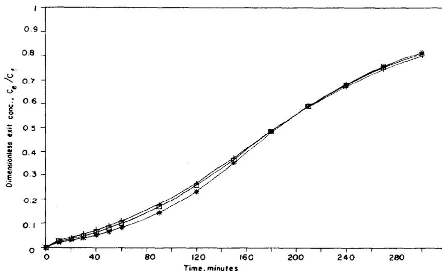
Fig. 5. Sensitivity analysis: effect of the solid-phase mixing coefficient  $E_s$  on the breakthrough curve;  $+0.3E_s$ ,  $\square$   $1.0E_s$ ,  $*$   $3.0E_s$ .
