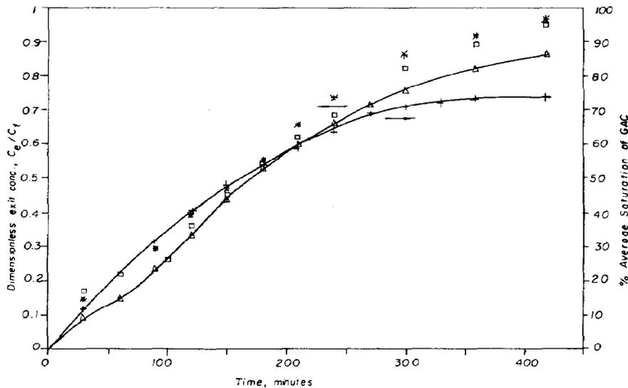
Fig. 10. Fluidized-bed adsorber breakthrough curve with 0.08 kg of  $1.545 \times 10^{-3}$  m  $\phi$  (# 12/14 mesh) GAC: \* experiment with  $C_f = 1.93$  mol/m<sup>3</sup>,  $\bar{u} = 0.0122$  m/s;  $\square$  experiment with  $C_f = 1.95$  mol/m<sup>3</sup>,  $\bar{u} = 0.0115$  m/s;  $\triangle$  simulation with  $C_f = 1.94$  mol/m<sup>3</sup>,  $\bar{u} = 0.0118$  m/s.
