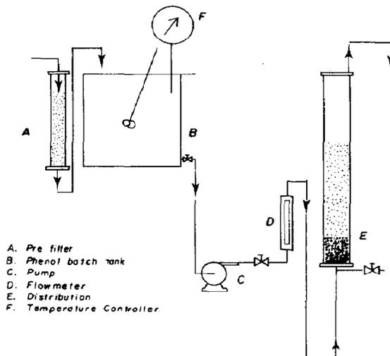
Fig. 8. Schematic of the experimental set-up.
