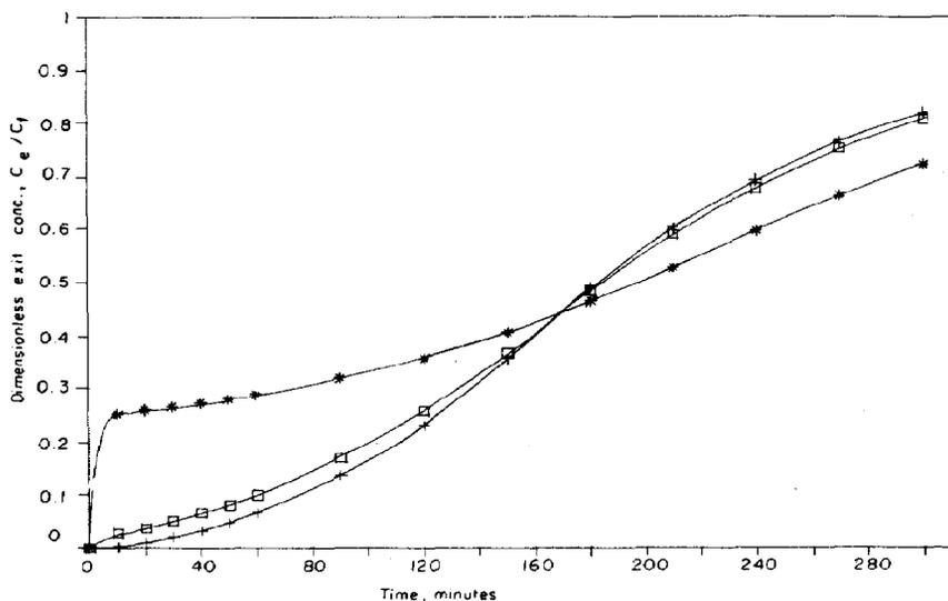
Fig. 4. Sensitivity analysis: effect of the external film mass transfer coefficient  $k_f$  on the breakthrough curve; \* $0.3k_f$ ,  $\square$   $1.0k_f$ ,  $\times$   $3.0k_f$ .
