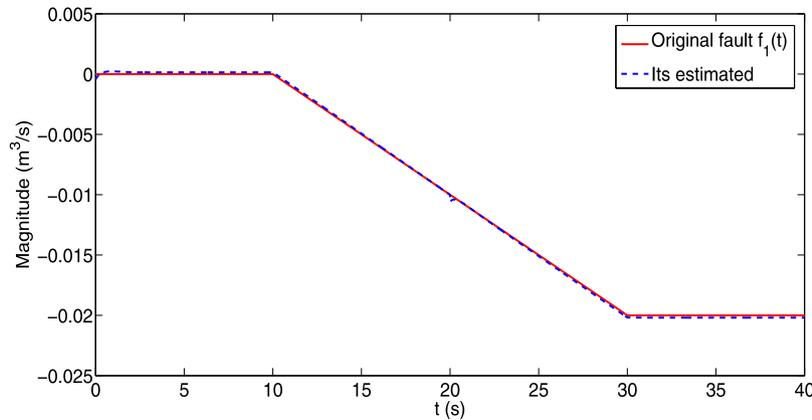
**Fig. 7.** The real actuator fault  $f_1(t)$  and its estimate given by the developed APO.
