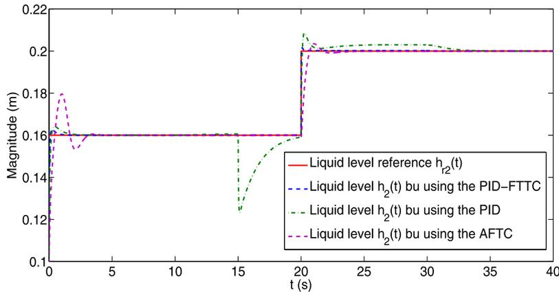
Fig. 6. Different comparisons of reference tracking  $h_{r2}(t)$  with the real liquid level  $h_2(t)$  by using the PID-FTTC, an AFTC and also a PID controller.
