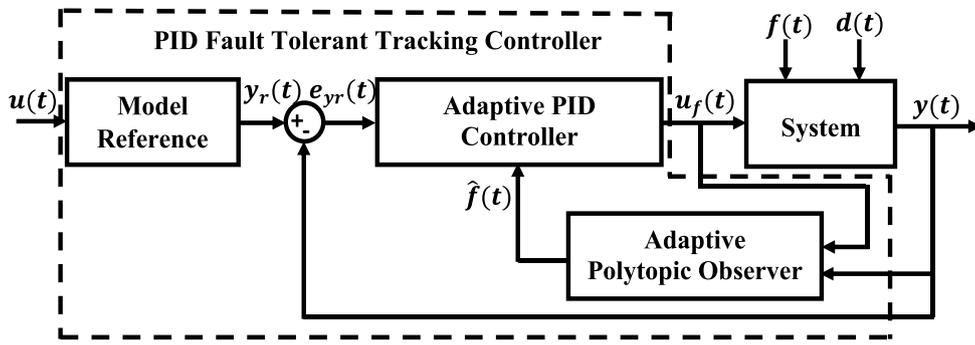
Fig. 1. PID Fault Tolerant Tracking Controller scheme.
