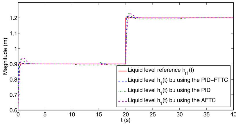
Fig. 5. Different comparisons of reference tracking  $h_{r1}(t)$  with the real liquid level  $h_1(t)$  by using the PID-FTTC, an AFTC and also a PID controller.
