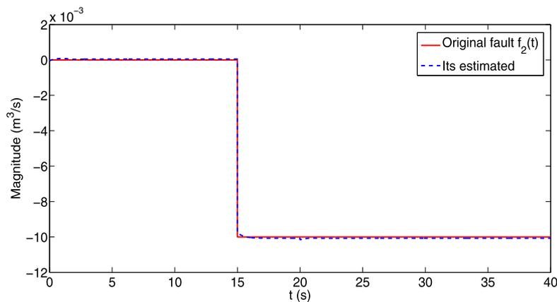
**Fig. 8.** The real actuator fault  $f_2(t)$  and its estimate given by the developed APO.
