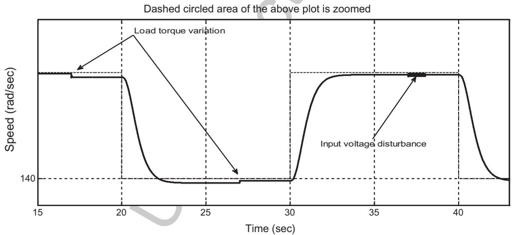
Fig. 6. The tracking performance of the adaptive fuzzy MIMO method [28].
