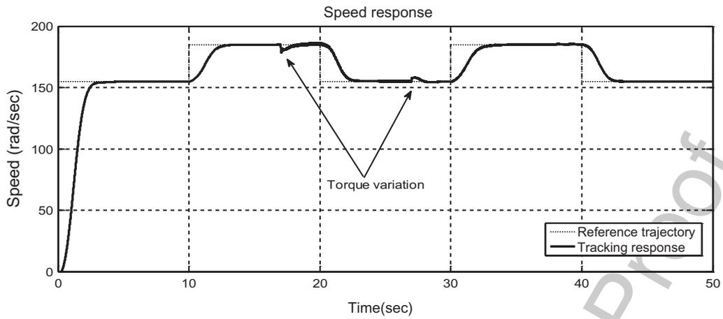
Fig. 5. The tracking performance of the proposed control scheme for the IM model described in Table 3.
