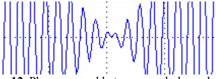
**Figure 12.** Phase reversal between symbols modulation
