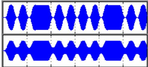
**Figure 9.** Gen 2 DSB modulation
