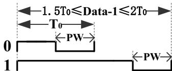
Figure 3. Gen 2 Forward link PIE encoding
