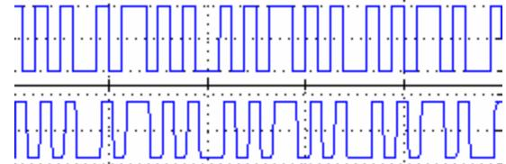
**Figure 16.** Gen 2 Miller subcarrier demodulation
