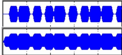
**Figure 8.** Class 1 PIE Modulation
