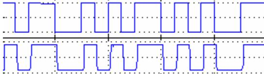
**Figure 15.** Gen 2 FM0 encoding demodulation
