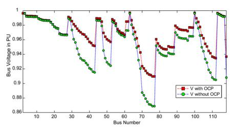
Fig. 6 Bus voltage profile of a 118-bus radial distribution feeder with and without OCP at full load
