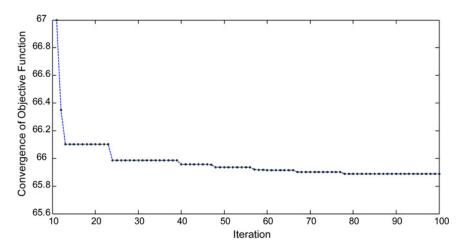
Fig. 4 Convergence trend of the objective for the case of a 69-bus loss minimisation
