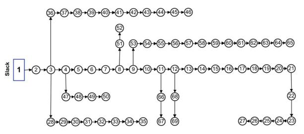
Fig. 2 One-line diagram of a 69-bus test radial distribution system
