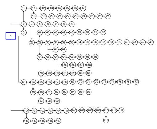
Fig. 5 Single-line diagram of the 118-bus radial distribution system (the bus number is reordered)
