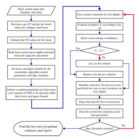
Fig. 1 Flowchart of CSA-based algorithm and capacitor allocations
