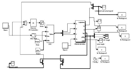
Figure 6 Simulation model of direct torque controlled PMSM
