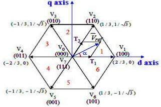
Figure 6 Basic switching vectors and sectors
