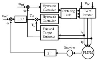
Figure 2 Block diagram of conventional DTC based PMSM
