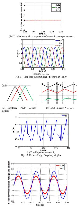
Fig. 13. Secondary voltages and currents
