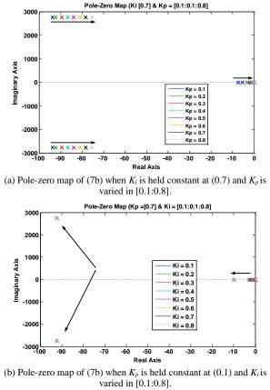
Fig. 7. Root loci for a fixed  $K_i$  and a range of  $K_p$  or vice versa.
