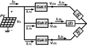
Fig. 2. Proposed Cuk-based three-phase Inverter
