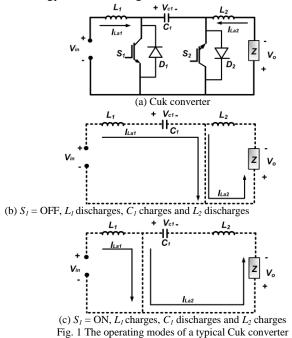
The state space averaging method will be used to model the Cuk converter. Assuming the turn off time of  $S_I$  is  $T_{off}$ , turn on time for  $S_I = ON$  is  $T_{on}$  and  $T_s = T_{on} + T_{off}$ , the state space equations during a continuous conduction mode of operation can be written as:
