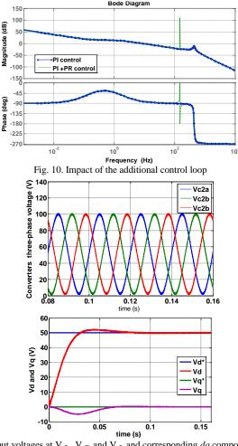
(a) Output voltages at  $V_{c2a}$ ,  $V_{c2b}$  and  $V_{c2c}$  and corresponding dq components
