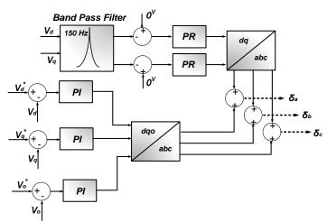
Fig. 9. Control structure with eliminating the  $3^{rd}$  harmonic in the dq frame ( $2^{nd}$  in the stationary)
