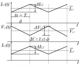
Fig. 3. Cuk converter operation
