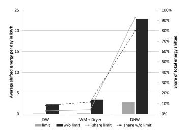
Fig. 6. Share of devices on shifted load without limit.
