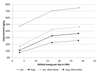
Fig. 5. Relation between shifted energy and improvement Aging, 20 kVA.
