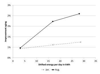
Fig. 4. Relation between shifted energy and improvement Aging, 80 kVA
