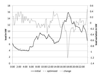
Fig. 1. Average daily load curve January, 10 households, max. 3.5 kWh shifted Energy.
